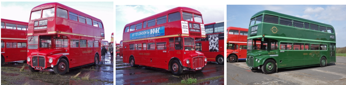
Standard RM Routemaster 27'6" long. RMLs were 30' with extra windows. Country and Green Line RCLs had doors.
